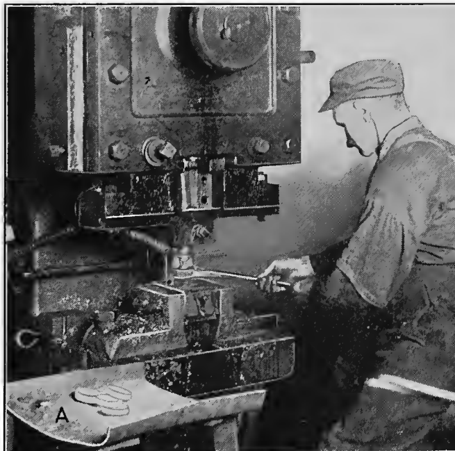
FIG. 3. DEEPENING THE DISKS
